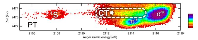
Figure 1: 2D map of S  $KL_{2,3}L_{2,3}$  Auger spectra of PT. White dashed line stadium-shape highlights CT region.
